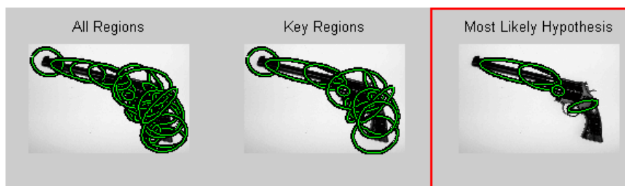
Figure 9: The images depict the flow of the recognition process. The image on the left shows the output from the IBR region detector. The middle image shows the 16 key regions after running k-means. The image on the right shows a gun being recognized, and the distribution of parts in the most likely hypothesis in the image.
